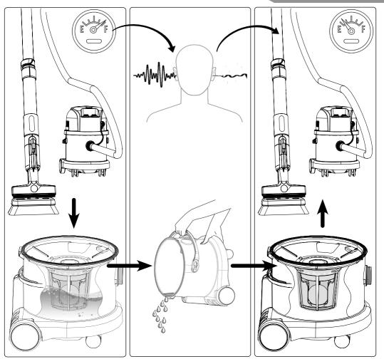
After cleaning the desired area, with the vacuum still running, collapse the wand and dock on the back of the CTB before turning the vacuum motor off.
